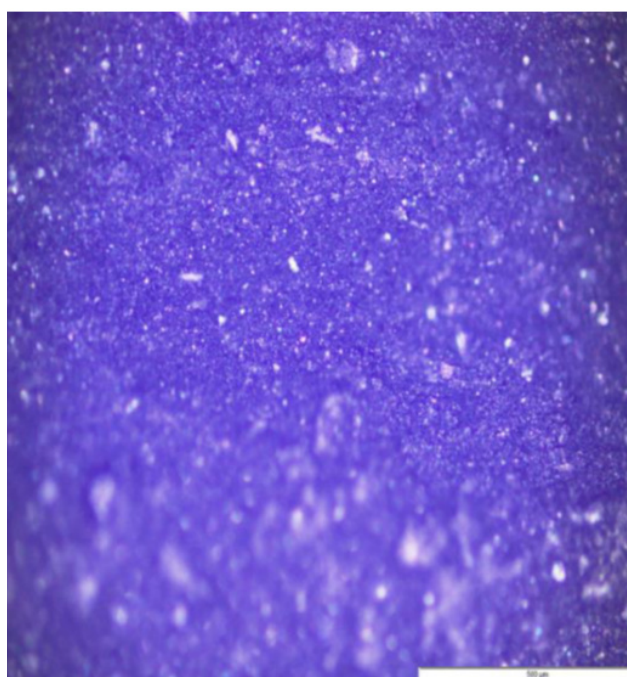
Figure 13(b): Micrograph of 20 wt.% cenosphere filled GJJG composite at load 20N
