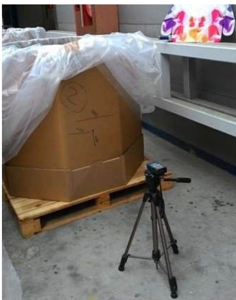
Figure 3. Measurement of the lateral deformations, \delta , of a point on the wall of the box.
