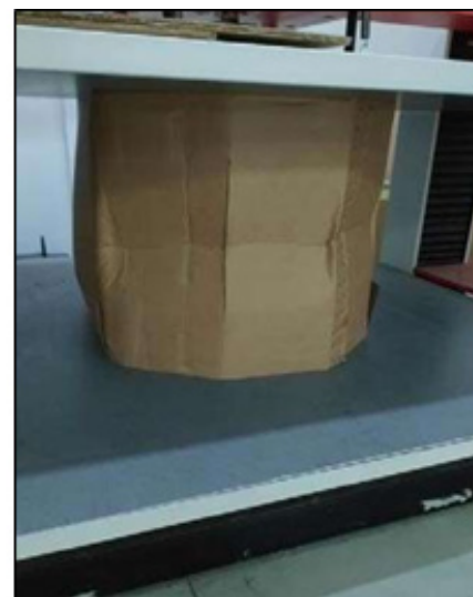
Figure 6. Images of the octabin in CAE simulation and in the testing machine.
