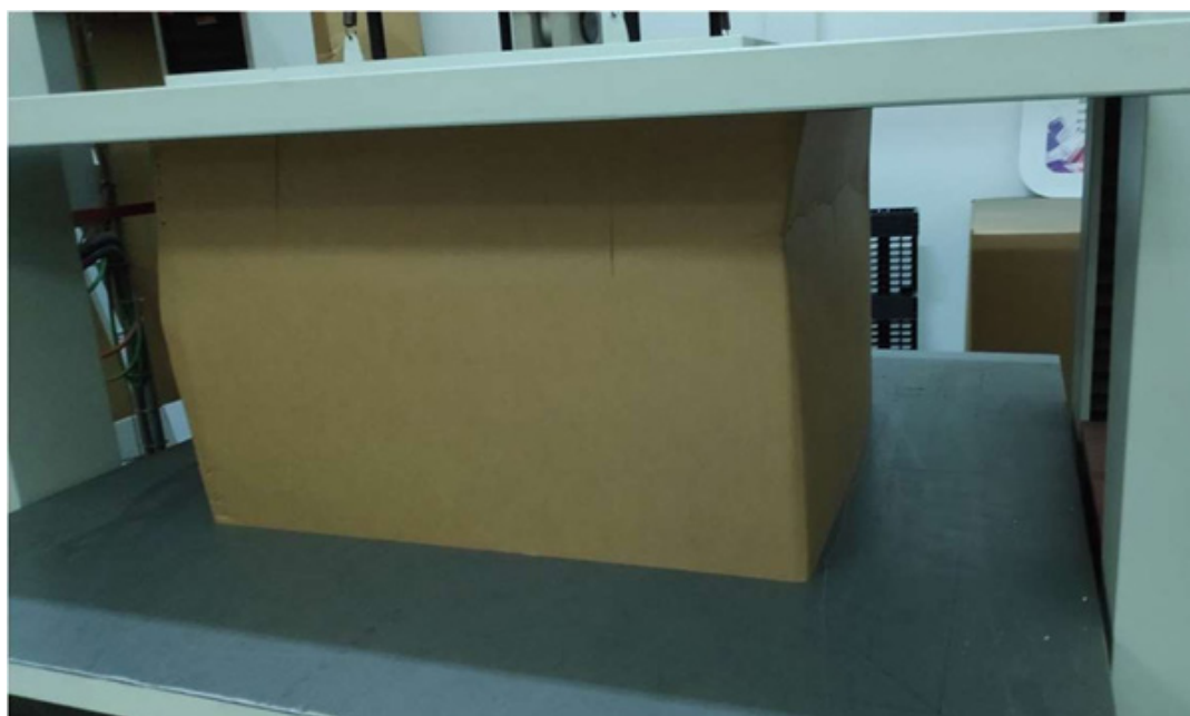
Figure 2. Compression Test (BCT) on corrugated card board boxes.
